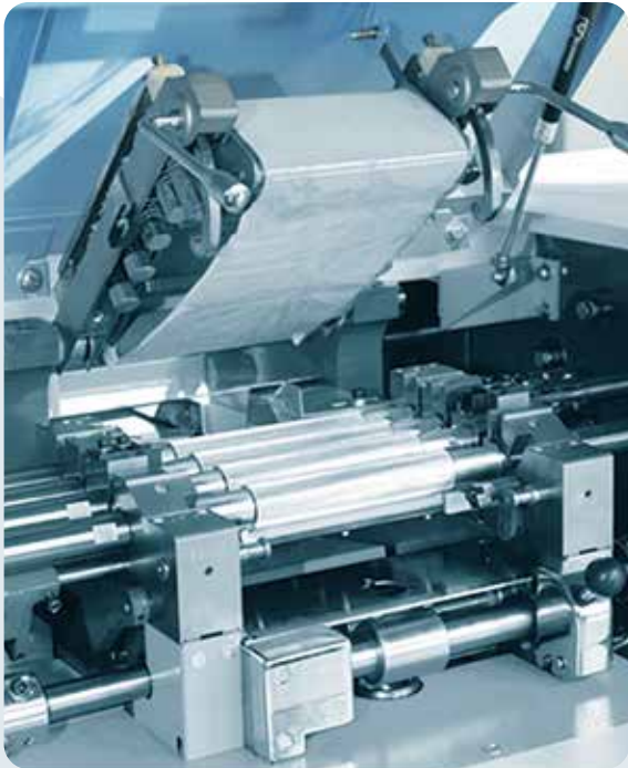
↑ 牵伸结构 Drafting structure
